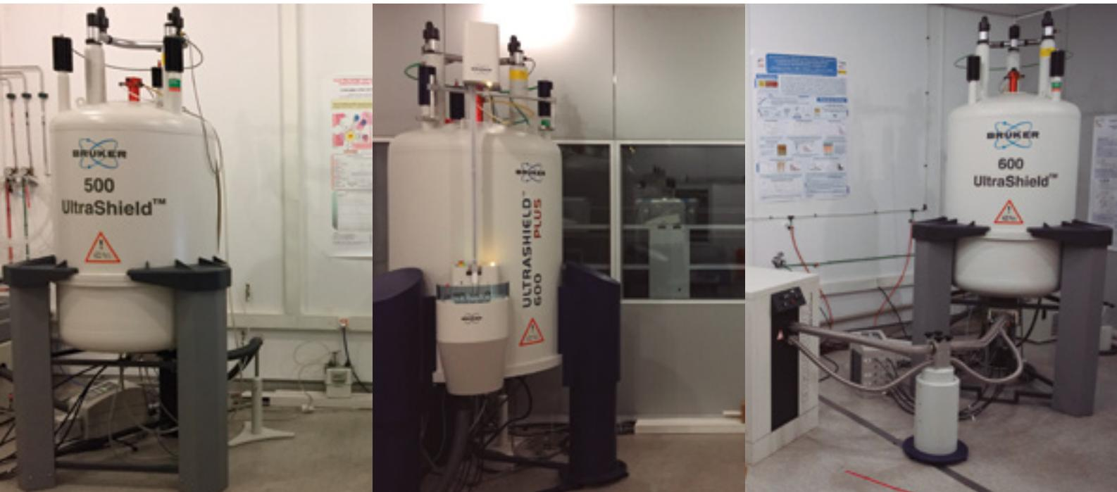
Technical Equipment of the NMR Service. From left to right: AV 500 MHz, AV III 600MHz, with Sample Case for 24 samples, and AV 600MHz with cryoprobe.
