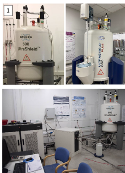
(1) Technical Equipment available at the NMR Facility. From top to bottom: AV 500 MHz (left), AV III 600MHz with Sample Case for 24 samples (right) and AV 600MHz with cryoprobe. (2) Example of DOSY (Diffusion Ordered Spectroscopy) of glucose (blue); maltose, a disaccharide formed by two glucose units (violet), and maltotriose, a trisaccharide of three glucose molecules (green).
