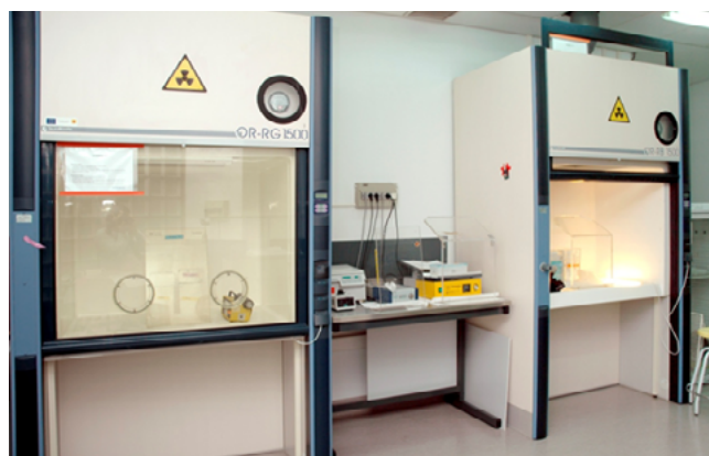
Central hot room: specific areas for manipulation of \beta and \gamma emitters.
